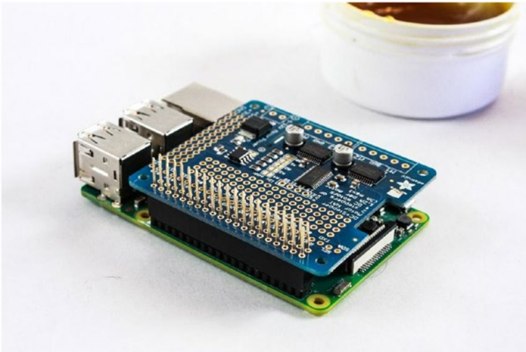
Figure 6-7. Circuit board mounted on the header
