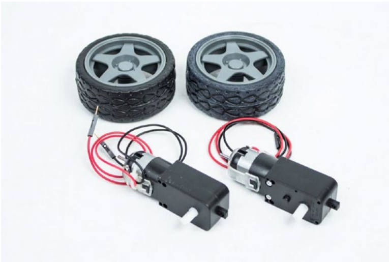
Figure 1-8. DC geared motor and wheels
