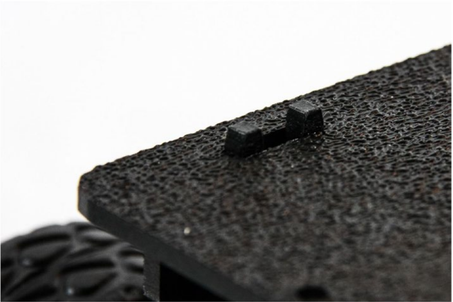
Figure 7-11. Clip protruding from the top plate
