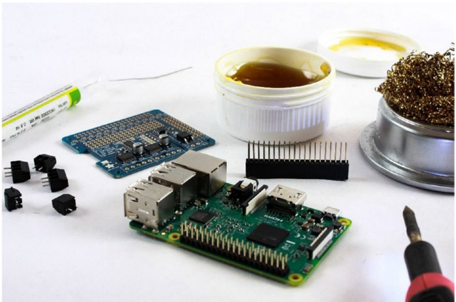
Figure 6-5. Preparing to assemble the motor HAT
